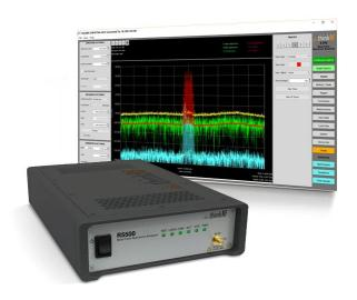
Along with this enhanced usability, the S240 software has introduced more measurement capabilities, including occupied bandwidth, zero-span mode and calibrated time-domain data. Features such as signal capturing, triggering and cursors have all been improved to enable better analysis, and frequently used settings can be saved to make setup more efficient.
